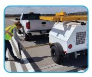
1. Level as necessary using 3 leveling jacks
