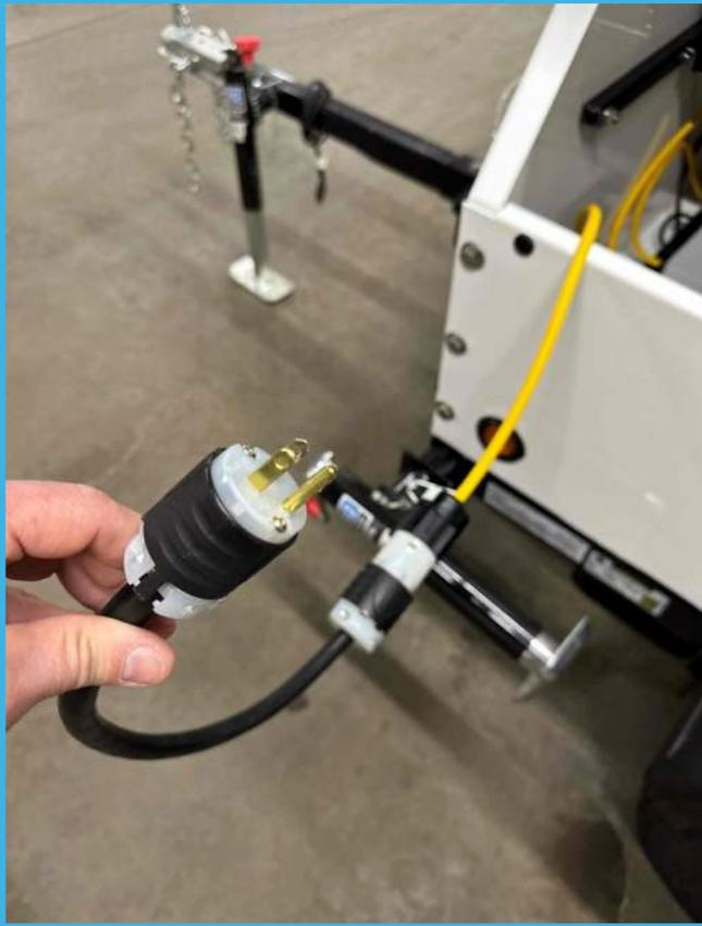
RCM adapter cord for shore power applications. 2' cord adapts lighted "x" plug so it can be plugged directly into any standard 120v, 15 or 20amp power outlet
