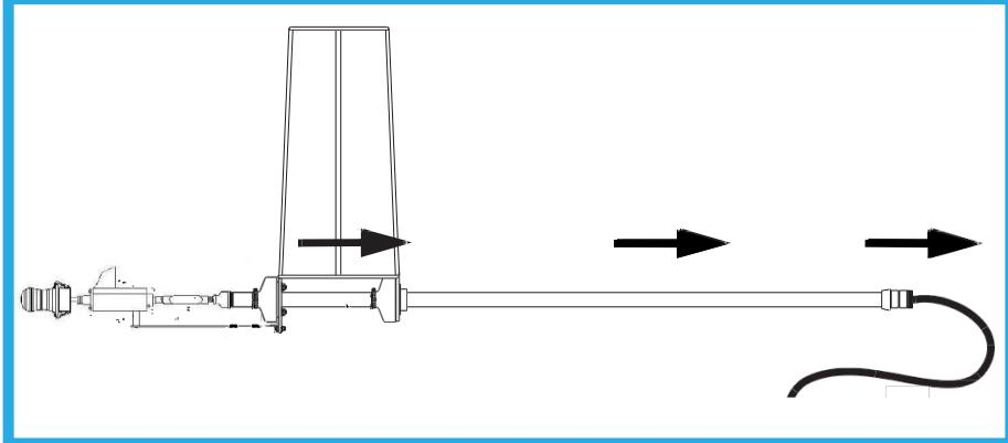
2. Push the wire cable through the basket support pipe and down the pole, out through the bottom
