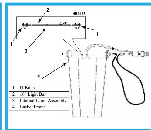
4. For external light kits, secure the Light Support bracket to the upper bracket and lower bracket attachments
